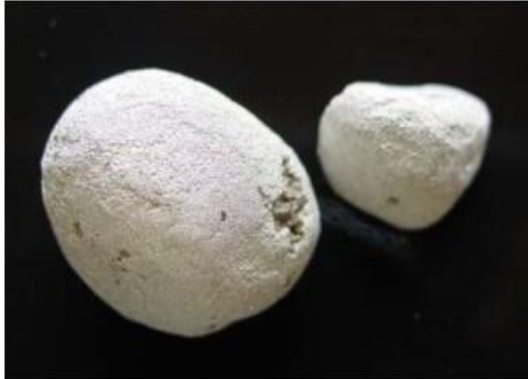
Two small clumps of mercury amalgam recovered from the wreck of the Atocha in 1984. They have a granulated texture and are quite soft.
